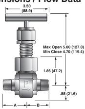
Panel Hole Diameter: 1.02 (25.9) Max Panel Thickness: 0.62 (15.7)
