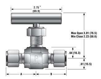
Panel Hole Diameter: 0.77 (19.6) Max Panel Thickness: 0.40 (10.2)
