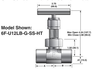
Panel Hole Diameter: 0.83 (21.1) Max Panel Thickness: 0.61 (15.5)
